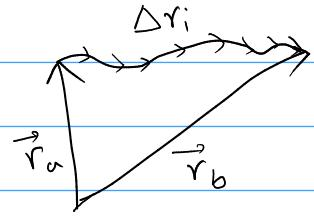
$$\int_{\vec{r}_a}^{\vec{r}_b} \vec{F}(\vec{r}) \cdot d\vec{r} = \int_{t_a}^{t_b} \frac{m}{2} \frac{d}{dt} (v^2) dt$$
